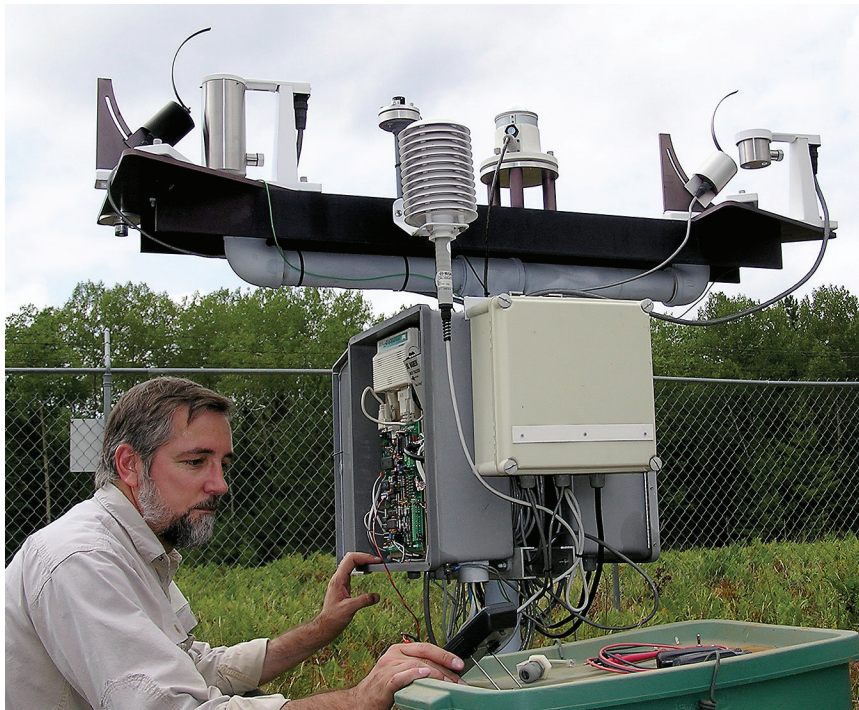
UVMRP field technician George Janson evaluating the electronic performance of the datalogger at the network monitoring site at University of Michigan Biological Station at Douglas Lake, MI.
