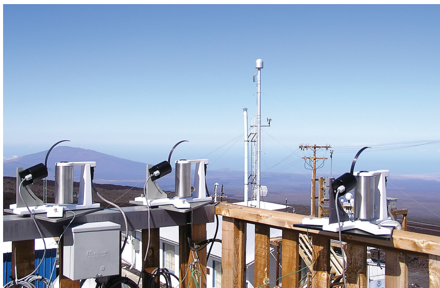
Three UV-MFRSR instruments occupy the UVMRP's intercomparison calibration site at NOAA's Mauna Loa Observatory on the Big Island of Hawaii. MLO is a world-renowned facility used by many atmospheric researchers for similar calibration of their instruments, due to the high altitude and clear air found at this location.
